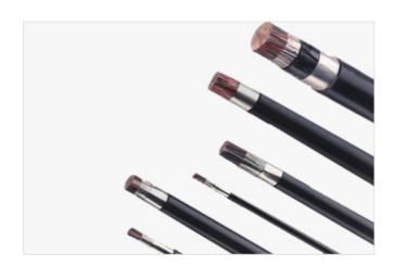
Polyethylene insulated jelly filled Telephone Cables are widely used for primary and Secondary distribution networks. The cables having single jacket are use as duct cables up to 2400 pairs as primary network. Secondary cables are directly buried and may Armoured with additional jacket of a tough weather resistance LDPE Compound.
