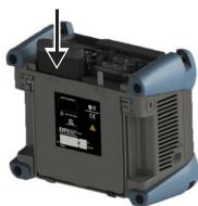
Place the battery compartment door on the unit so that it is flush with the top and back of the unit. If necessary, slightly move the battery compartment door until alignment is correct.
