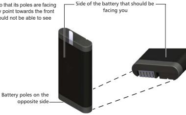
Slide in the new battery, and push it toward the bottom of the unit until it stops.
