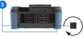
4 Remove the battery compartment door.
