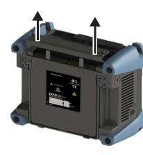
Use the markings on the back panel to locate the battery that you want to replace, and then pull on the battery's tab to free it from its socket.
