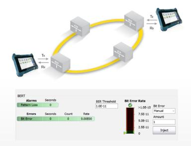
The multiple MAX-800 models offer the ability to preconfigure bit-error-rate (BER) thresholds that are user-defined prior to running the test, thereby generating a simple pass/fail verdict at the conclusion of test to overcome misinterpretation of test results.
