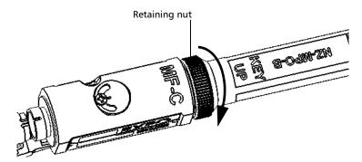
**4.** Insert the inspection tip on the MF-Ready probe by aligning the key of the probe with the notch of the inspection tip.
