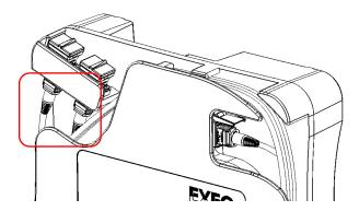
**4.** Open the dust cap and connect the DUT to the appropriate adapter according to the connections you made at step 3. If you have connected an MPO-24 split patchcord, you will have to connect the DUT, in turn, to each of the two adapters.
