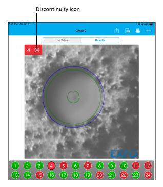
A fail status either on the inspection of the connector, the polarity or continuity will result in a global fail status.
