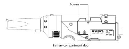
**4.** Remove the battery compartment door.
