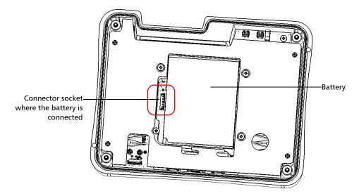
**Note:** To simplify the illustration, the battery cable and several other components do not appear.
