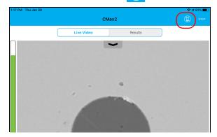
**2.** As soon as a the status LED displays a pass or fail status, press the Fiber Inspection Probe capture control button to perform another inspection.
