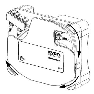
**3.** If you are using a patchcord having a single MPO-12 or MPO-24 connector, you can connect it to any of the two adapters. With an MPO-24 split (Y) patchcord, you must connect each of its ends to one of the adapters.
