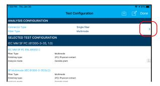
**6c.** In the **Analysis Configuration** window, tap > to change the connector type.
