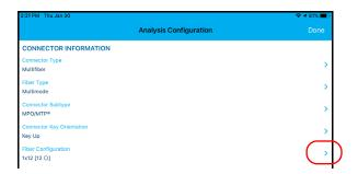
**10b.** Select the fiber configuration applying to the connector you use for your inspection.
