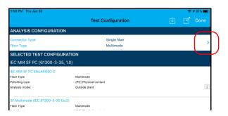
**5c.** In the **Analysis Configuration** window, tap > to change the connector type.
