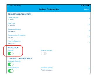
**12.** To determine on which fibers the discontinuities are found, activate the option. See *Understanding Fiber Continuity* on page 108 for details.
