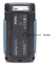
**4.** Remove the battery compartment door.
