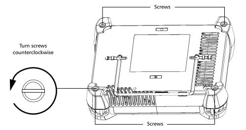
**4.** While holding the front and the back panels firmly together, turn the unit over, and position it so that its *back* panel rests on a flat surface such as a table.
