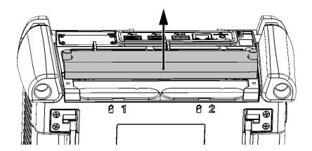
**2.** Use the markings on the back panel to locate the battery that you want to replace, and then pull on the battery's tab to free it from its socket.
