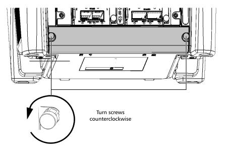
**1c.** Remove the battery compartment door.
