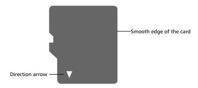
**3.** Slide the card into the unit's microSD card slot, and push it all the way to the bottom of the card slot.
