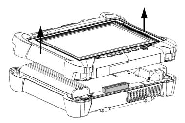
**6.** If you are working with a MAX-860 unit, pull up the battery filler to remove it and expose the battery.
