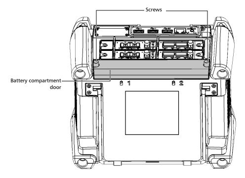
**1b.** Turn the battery compartment screws counterclockwise until the compartment door is loose. Since they are captive screws, you cannot remove them completely.
