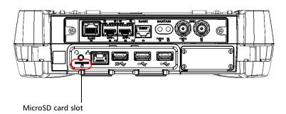
**2.** Pull the card out of the unit's microSD card slot.
