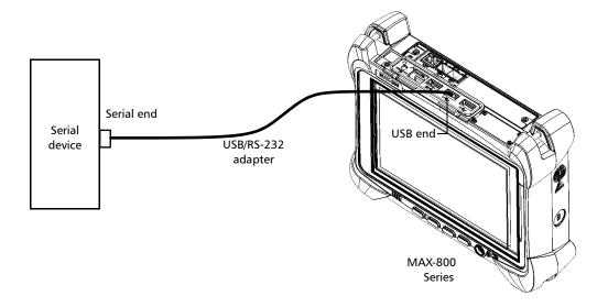
**Note:** If the device that you want to use is a computer (not equipped with USB ports) you may want to use a null-modem serial cable as an "extension cable" between the device and the USB/RS-232 adapter.
