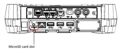
**2.** Position the card vertically so that its smooth edge is on the right and you do not see its gold area. If an arrow is printed on your card, it should point toward the bottom.
