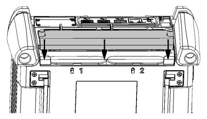
**7.** Turn the battery compartment screws clockwise until they are tightened.
