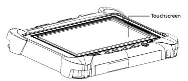
**5.** Place the front panel on the back panel of the unit, making sure that the mating connector of the back panel is aligned properly with the corresponding slot on the front. The bumpers of the back panel should be flush with those of the front. If necessary, slightly move the front panel until alignment is correct.
