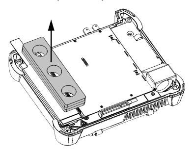
**7.** Pull on the battery's tab to free it from its socket.
