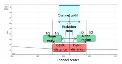
OSNR distance (GHz or nm): Except for the fifth order polyfit selection, the OSNR distance is automatically set at the channel edge, that is, at half of the channel width from the center wavelength.
