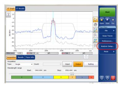
Setting Up Spectral Transmittance Analysis Parameters
