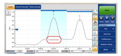
A dotted line across the full spectral width corresponds to the peak detection level indicator. This line indicates the minimum power level (dBm) from where a peak can be considered as a valid signal.
