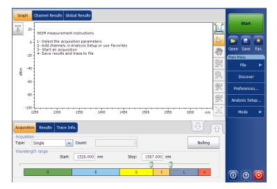
When the acquisition is taken (see *Starting a Measurement* on page 237 for details on how to perform a test), the active trace will be displayed in the tab with information along the following axis values:
