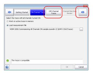
**6.** Using the buttons at the bottom of the window, select all of the applicable measurements traces (files) with one corresponding channel off. An indicator next to the trace shows if the measurement file is compatible or not.
