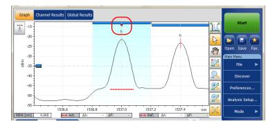
The noise level for a channel is indicated by a dotted line under the selected peak. The width of the noise level indicator is set according to the current Noise for OSNR setting. The width of the noise level indicator depends on the noise associated with the OSNR setting (from the largest to the narrowest): IEC, InB, InB nf and fit.
