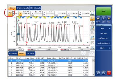
**2.** Set the marker by entering precise values in the box corresponding to it or by dragging it on-screen.
