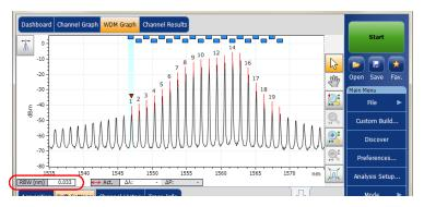
The graph will display peak indicators for all the channels found by the application with a red vertical line over the peaks to indicate the peak position.
