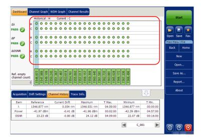
The dashboard shows a global status (all channels) for each parameter. This global status is set to Fail if at least one channel has a failed historical status for that given parameter, otherwise the global status is set to Pass.
