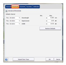
**3.** Select the **Activate all thresholds** option to manually set the channel threshold values. If this option is not selected, all the thresholds will be deactivated, results are displayed without a Pass/Fail status in the **Channel Graph**, **Channel History** and **Channel Results** tabs.
